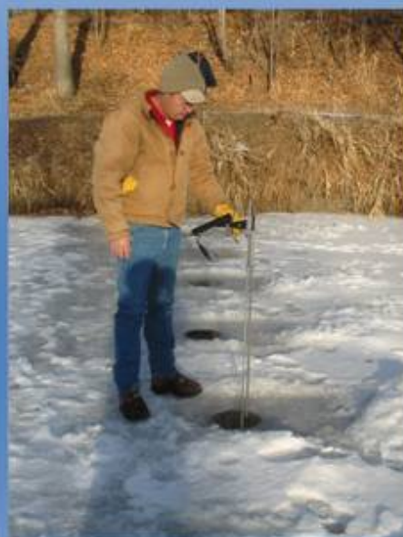
Discharge measurements can be made through the ice by drilling a transect of holes. Under-ice flow rating curves will differ from open water rating curves due to friction from the ice.
